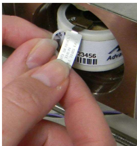
Figure 8. Inserting sensor in cell block
