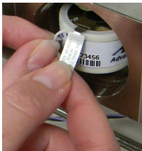
Figure 8. Inserting sensor in cell block
