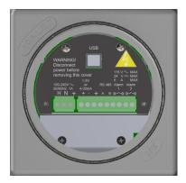
The green terminal block connectors are combination connectors, which allows you to unplug
