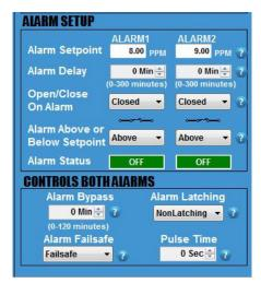
The Analyzer features 2 independent  $\rm H_2S$  Concentration Alarms –one for ALARM 1 and one for ALARM 2. The settings for these alarms, including setpoints, relay contacts, close/open logic and alarm delays, are adjusted through the **COMMAND CENTER**.
