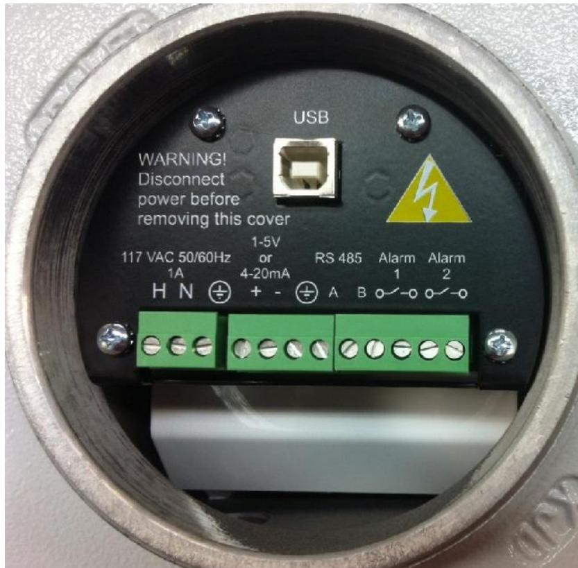
**Figure 3. Interconnections (AC unit shown)**
