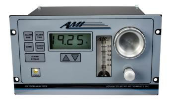
The AMI model 201RS is the ideal solution for measuring percent oxygen in a wide range of applications in a general purpose environment. In a compact size, and at low cost, it provides a comprehensive electronic package and sample system using AMI's patented cell block technology. In addition the 201RS uses internal surface mount solenoid valves for sample/span gas selection and to seal off the sensor in the event of loss of power.
