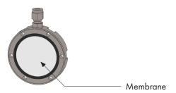
11) While holding the center of the membrane in place with one finger, align the Body O-ring with its groove and apply a slight amount of pressure in a 4-area pattern, making sure the membrane does not move during this process. While still holding the membrane in place with one finger, continue to press the Body O-ring in place until it is completely seated into the groove.
