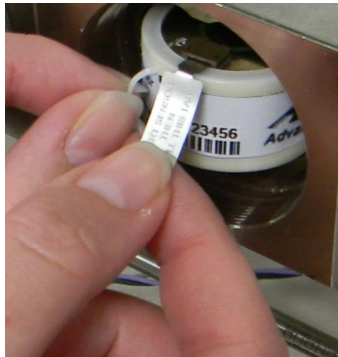
Figure 8. Inserting sensor in cell block
