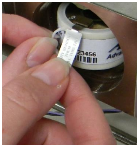
Figure 11. Inserting sensor in cell block
