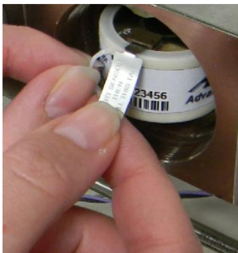
Figure 9. Inserting sensor in cell block
