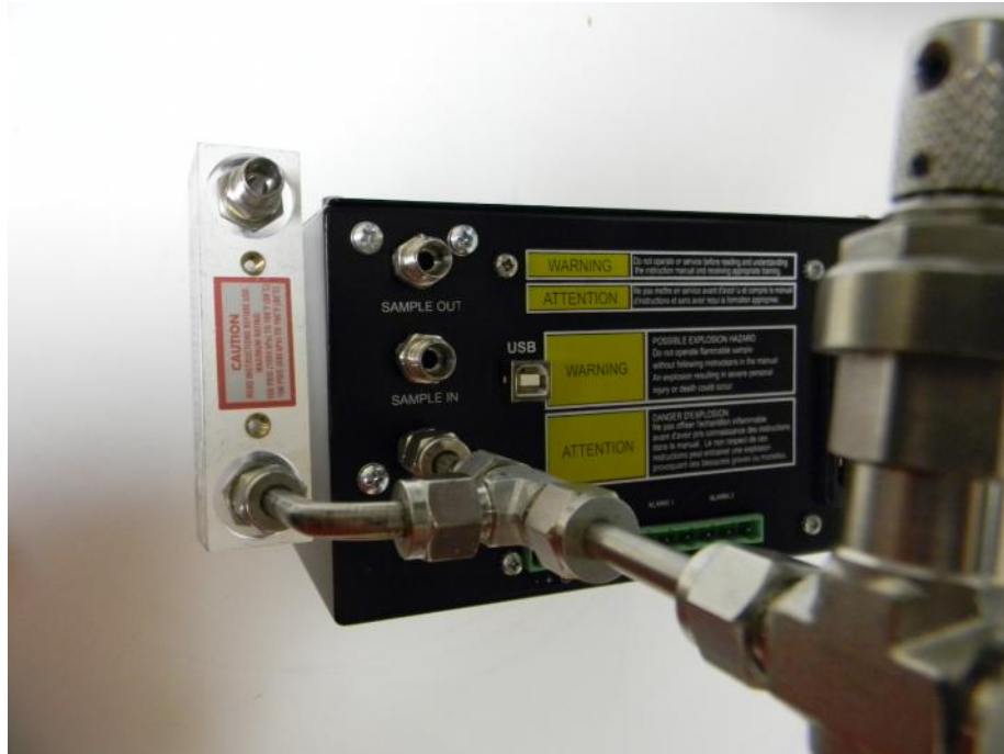
Figure 8 Span gas bypass connection – back view.
