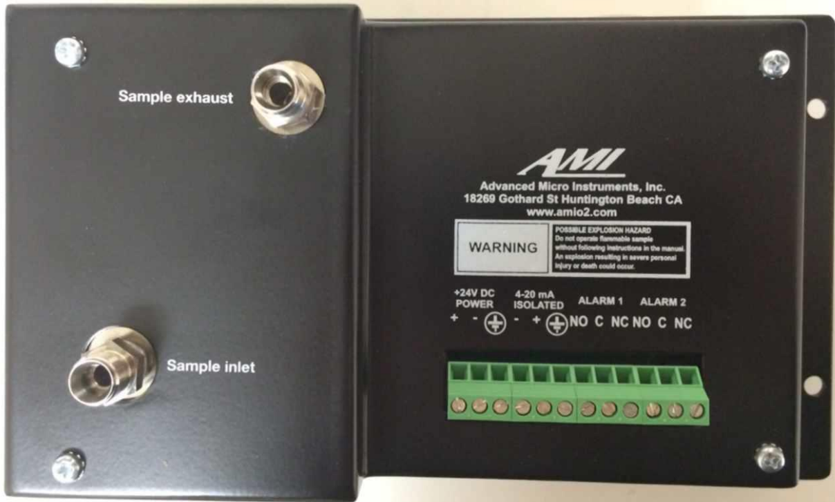
Figure 1. Back panel of 2001LC analyzer
