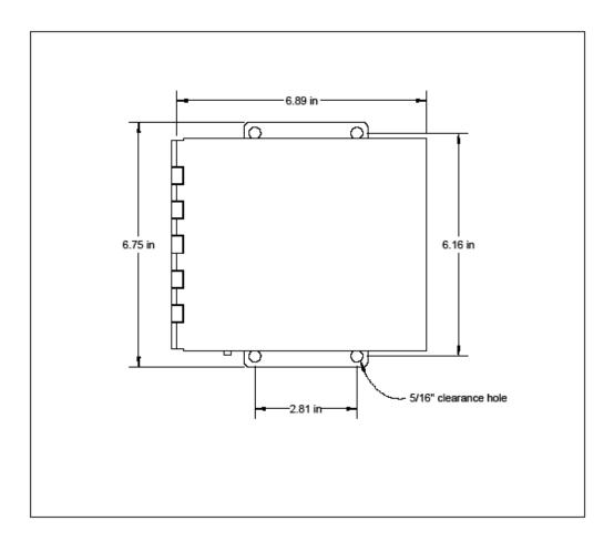
**Figure: Mounting Hole Dimensions**
