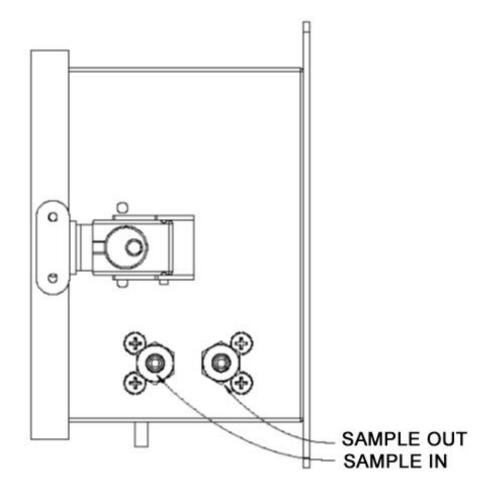
Figure: Plumbing Connection Illustration
